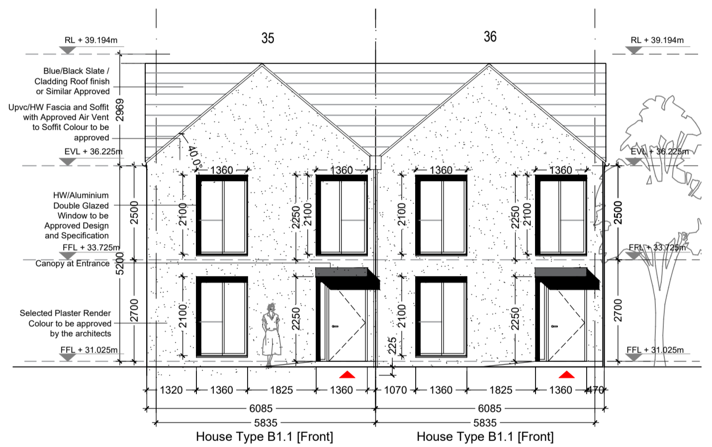
03 FRONT ELEVATION 1:100 BLOCK 12
