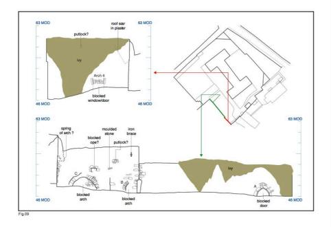
The middle section of wall F14 has several oolitic limestone blocks from the abbey (plate 13). The lower courses of this wall form a distinct horizon. In general the stonework of this wall is poor, with smaller triangular stones, roughly coursed, and notable chipped surface on the stone.
