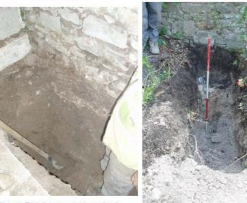
Plate 11. Trial pit 1, shovel at base of wall.
