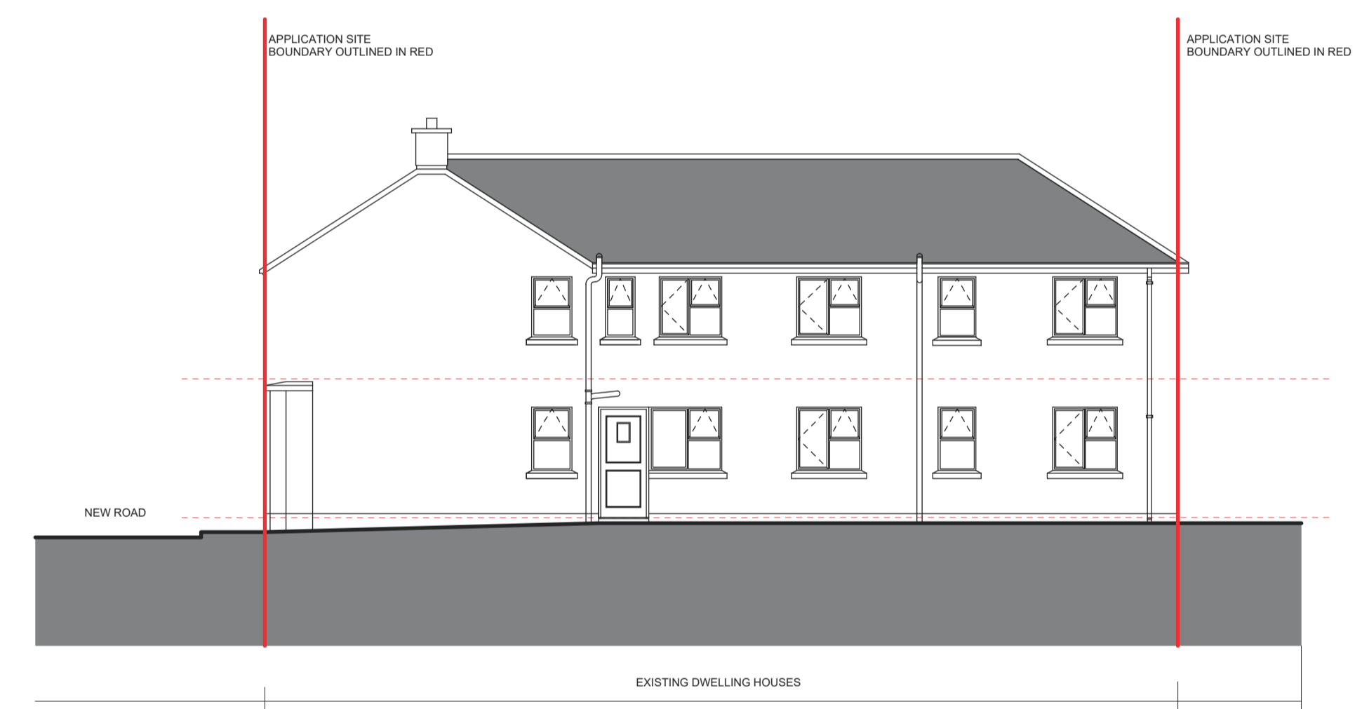
04 EXISTING SIDE ELEVATION 010 1:100 @ A1
