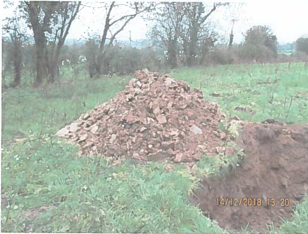
SOIL/SUBSOIL/COBBLES OF EXCAVATED TRIAL HOLE
