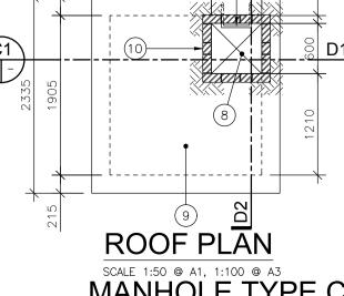
C1 SECTION MANHOLE TYPE C (BLOCKWORK) 1m ≤ DEPTH TO INVERT < 3m
