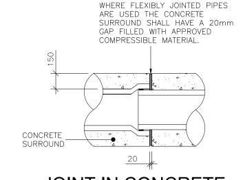
**CONCRETE PIPE ENCASEMENT DETAIL**
