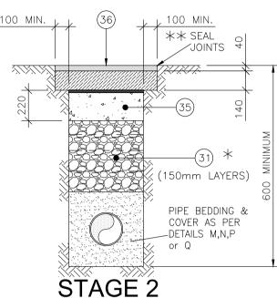
DIG OUT SURFACING & TOP 220mm OF CL804 MATERIAL (31) & REPLACE WITH NEW WIDER SURFACING ON 220 LAYER OF LEAN-MIX CONCRETE (35)
