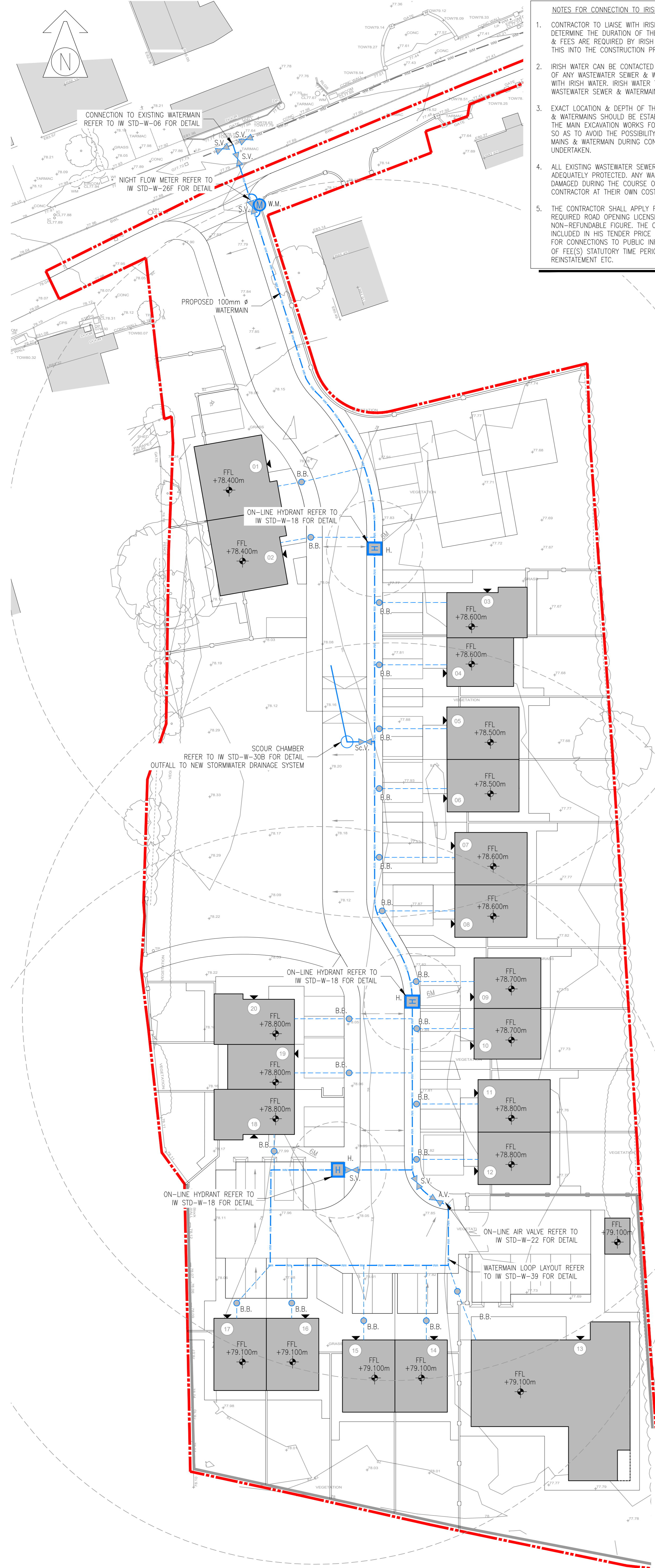
PROPOSED WATERMAIN LAYOUT SCALE 1:250 @ A1 / 1:500 @ A3
