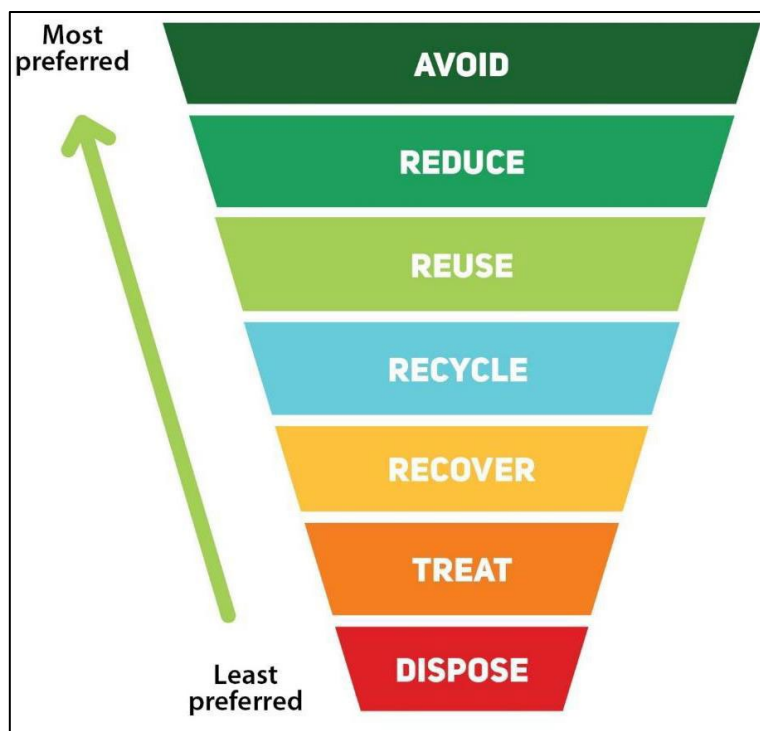
Figure 4.1: The Waste Hierarchy; The most preferred option is to prevent waste, and the least preferred choice is disposal in landfill sites.
